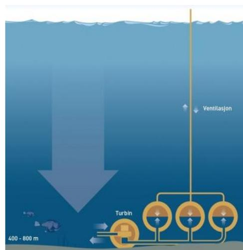
work by opening when energy is required. Water flows into the tanks turning a generator as they do so.
