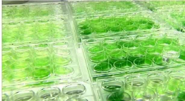
Scientists from Synthetic Genomics and ExxonMobil have solved this problem by developing a strain of algae that converts carbon into a record amount of energy-rich fat, which can then be processed into biodiesel or burnt to produce steam to spin turbines. 40% of the algae's mass is fat which is over double the fat content of conventional algae.
